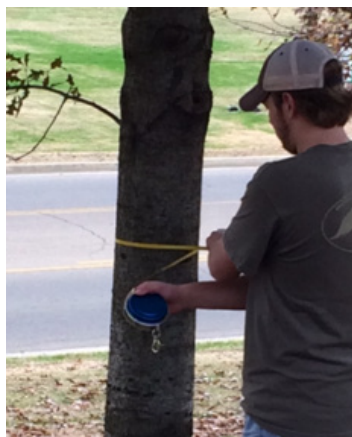
Using the diameter tape to measure DBH. Follow the correct procedure to hold the tape (Appendix 9).
