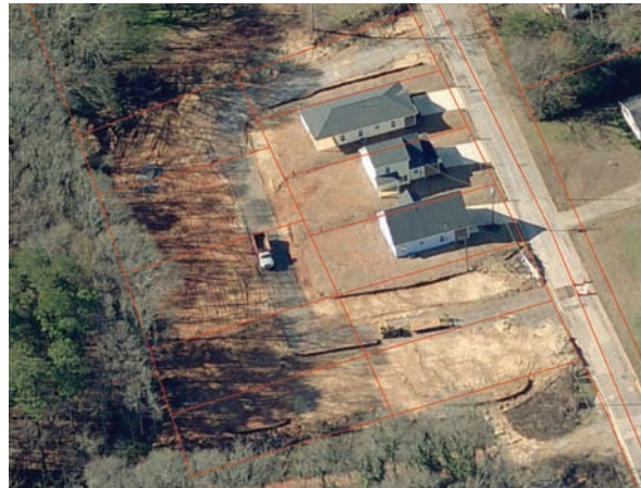
Figure 26 - These 12 lots were created in a series of four subdivisions to avoid basic site construction standards.
