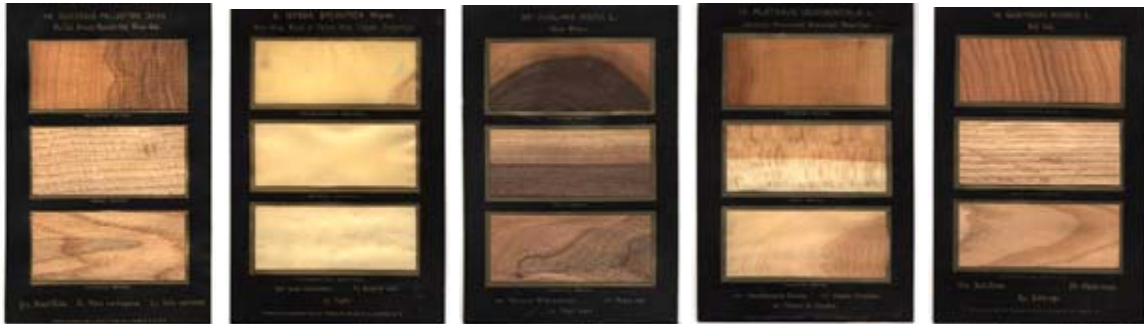
The three surfaces of some locally grown hardwoods (from left) Willow Oak, Black Gum, Black Walnut, Sycamore and Pecan.
