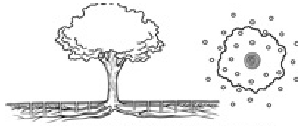
Figure 3. An Air Spade or Vertical Mulching Can Decompact Soils
