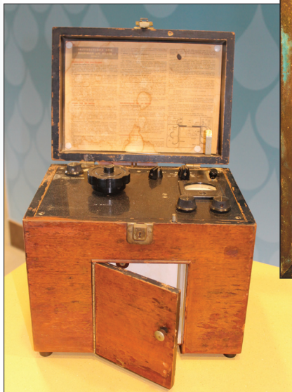
Left: The Beckman Model "G" pH meter was the first automated and portable laboratory instrument of its kind. Above: The federal Public Works Administration, one of President Franklin D. Roosevelt's New Deal programs, funded some of the filter equipment, a new raw water pumping station, additional distribution lines, and an elevated storage tank for the 1936 building.
