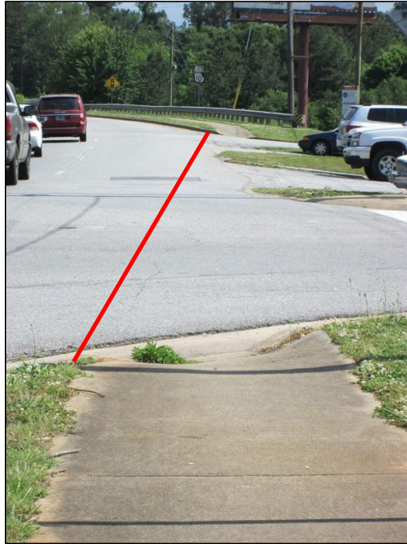
FIGURE 60. SIDEWALKS ACROSS S. HOMEWOOD DRIVE DO NOT ALIGN.
