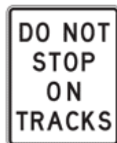
FIGURE 19. DO NOT STOP ON TRACKS (R8-8) SIGNS SHOULD BE USED WHERE SIDE STREETS CROSS RAILROAD TRACKS.
