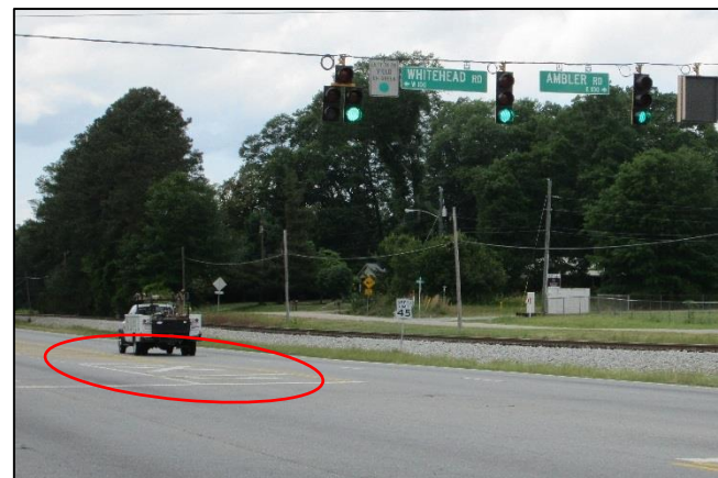
FIGURE 27. SHORT TURN LANES AND INSUFFICIENT LANE STORAGE FOR VEHICLES TURNING ONTO WHITEHEAD ROAD.
