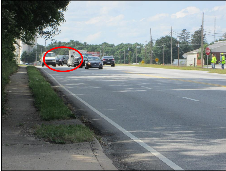
FIGURE 17. TYPICAL SCENE IN WHICH VEHICLES PULL INTO ADJACENT LANES TO GET AROUND THOSE WAITING TO TURN LEFT ONTO A SIDE STREET, SEEN HERE AT THE ENTRANCE TO THE KINDER MORGAN FACILITY.
