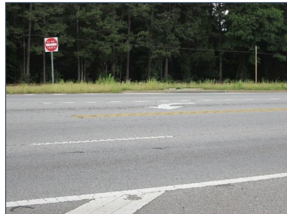
FIGURE 21. MISLEADING "DO NOT ENTER" SIGN FACING SOUTHBOUND DRIVERS NEAR LAVENDER ROAD.
