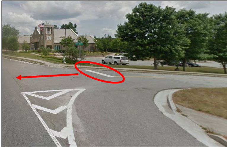
FIGURE 30. STOP BAR SET TOO FAR BACK ON FIREFIGHTER COURT.
