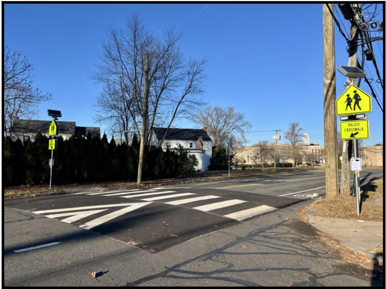
EXAMPLE OF MID-BLOCK CROSSING WITH LOW PROFILE RAISED CROSSWALK
